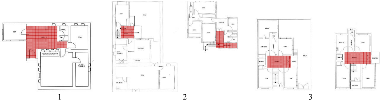
Fig 5. Plan types-houses with inner halls(1), inside and outside halls(2) and central halls(3) (Şenol, 2007)
