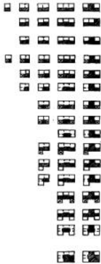
Fig 3. The Matrix of Planimetric Organizations of the 'Turkish house: the plan type with an outer sofa
