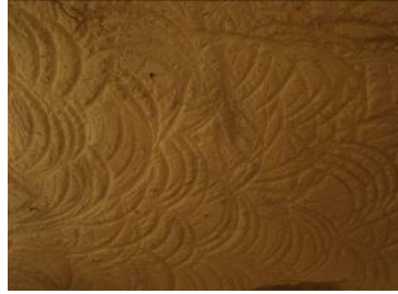
Fig. 5 The texture formed after the extraction of the big rock masses via machines
