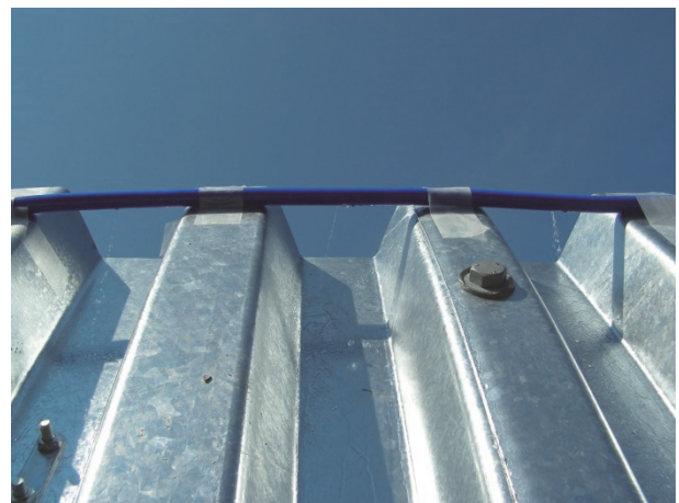
Figure 22. Water sprinkling experiment of plank sheets. We sprinkled 24-29°C tap water from the blue hose.
