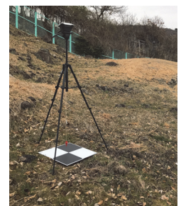
Fig. 4. GNSS survey of GCPs with Reach RS (taken on February 21, 2018)
