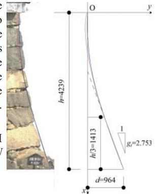
Figure 10. Curves of TS-L (right) and comparison with projection of photogrammetric result (left) S=1:100 (blue: GM, green: SS, red: IH). Width of projection (left) is  $\frac{\sqrt{3}}{2} \approx 0.866$  times that of actual *ishigaki*.
