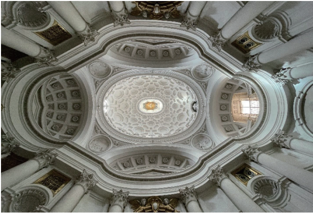
Fig 3. Upside view of the San Carlo Church. The entablature has the same wavy form as the plan. It surrounds the interior of the church, supported by 16 columns.
